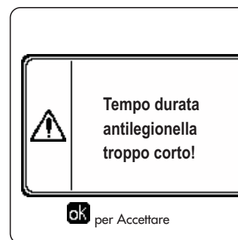
fig. 27- Message Anti-legionella function not completed
